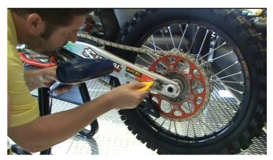
\* While heating in moderation, using Squeegee to press DeCal into the edge or fold over area. Allow DeCals to "set" for 48 hours before use
