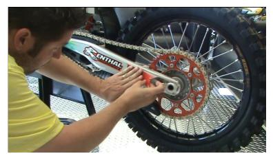
\*Applying DeCal to top edge of machined surface (Do not stick down entirely, yet)
