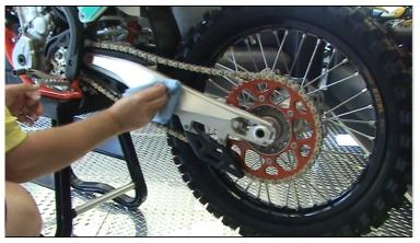
\*Using DeCal Works Step 1 and 2 fluids after swingarm has been throughly pressure washed etc. (Contact cleaner can be used as a de-greaser)
